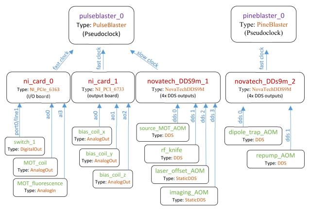
Here we see two PseudoclockDevice instances in the top tier of the diagram. They do not have a parent device that tells them when to update their output (this is true for all PseudoclockDevice instances). However, all but one (the master pseudoclock device) must be triggered by an output clocked by the master pseudoclock device.
